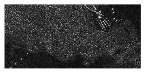
Figure 3: CARABAS-II (20-86 MHz) SAR image (2.5-m resolution). 25 vehicles of different sizes and orientations as well as a few buildings are clearly visible in the open field.
