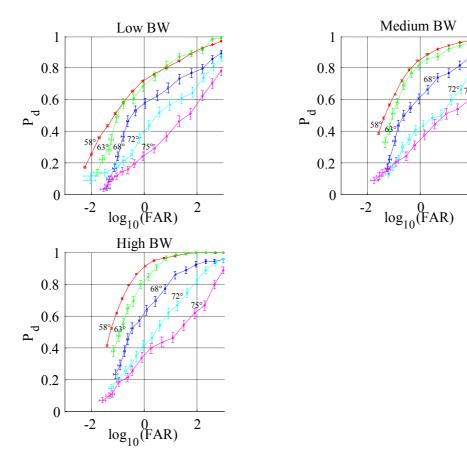
Figure 10: ROC curves for study two showing performance as a function of incidence angle for various bandwidths. The 58°, 63°, 68°, 72° and 75° incidence angle results were generated using 68, 4, 4, 4, and 4 image pairs, respectively. There were only 200 targets available for the 75°, 72°, 68° and 63° cases whereas the 58° case had 3400 target available. FAR is given in km<sup>-2</sup>.
