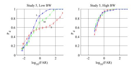
Figure 9: ROC curves for study one. Left: Low bandwidth (27-50 MHz); Right: High bandwidth (30-80 MHz). Legend: small (dash dot), medium (dash), and large (solid) targets. 23 image pairs were analyzed, including 460 small, 368 medium, and 322 large targets. FAR is in km<sup>-2</sup>.
